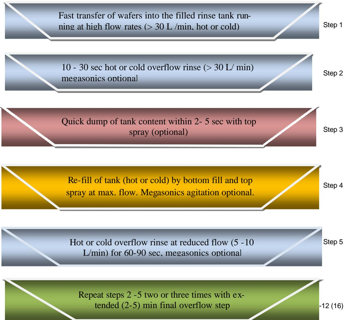
The table below provides an overview of typical parameters for each of the steps in a three cycle quick dump process as shown above. These might vary by customer and application, but serve well for setting up a general base process.
