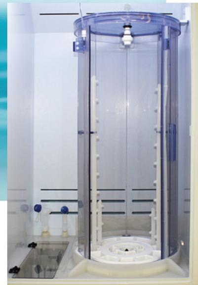
*The tube washing chamber contains a proprietary nozzle for conformal etch.*
