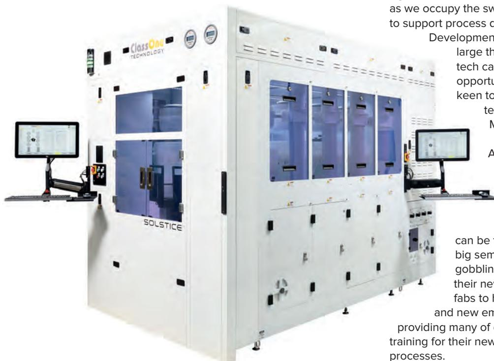
► Above: The ClassOne Solstice single-wafer platform provides advanced electroplating and wet process technology.
