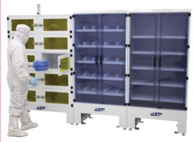
JST specializes in offering end-users with the capability to store work in process in a controlled environment. Features are provided specific to product storage requirements with emphasis on safe handling and organizational layout. Design construction of cabinet prevents contamination build up with sloped surfacing; ideal for the clean room environment.
